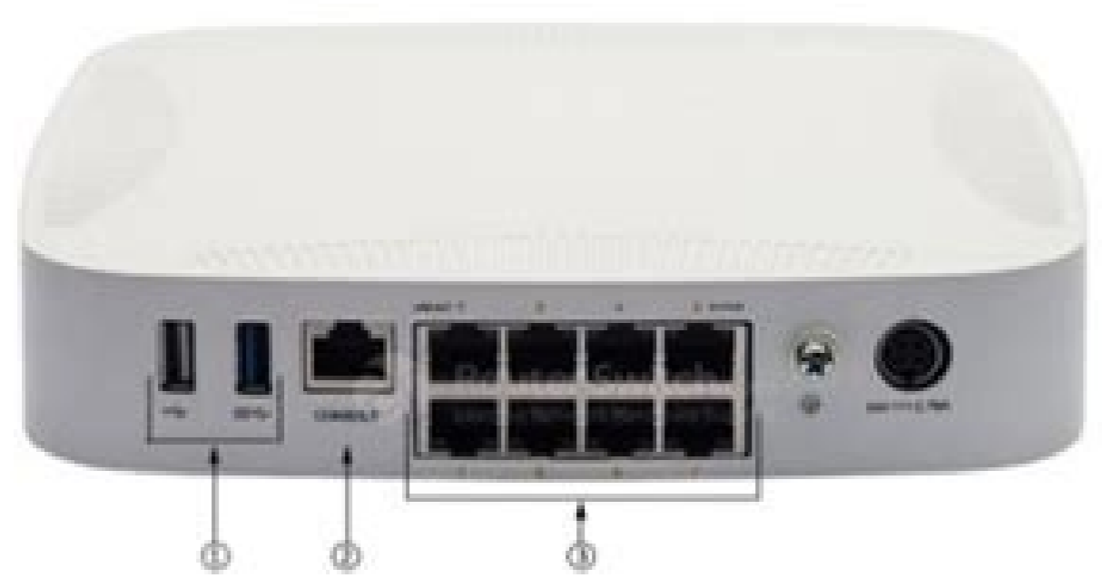
Figure 3 shows the ports of Aruba 7008 controller.
